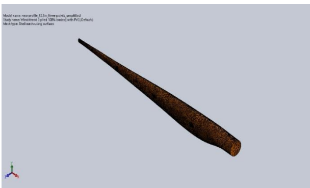
Figure 2.3: Meshed view of blade
